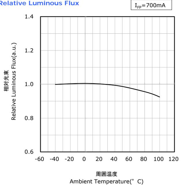
FORWARD CURRENT CHARACTERISTICS / TEMPERATURE CHARACTERISTICS
